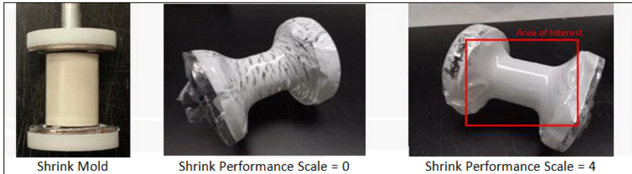
Figure 2– Shrink Mold and Performance Criteria
